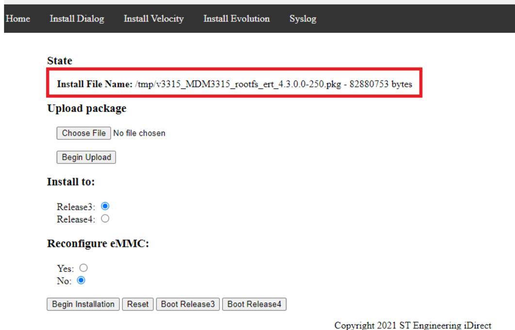
Figure C-6. Evolution Software Package Upload Confirmation
