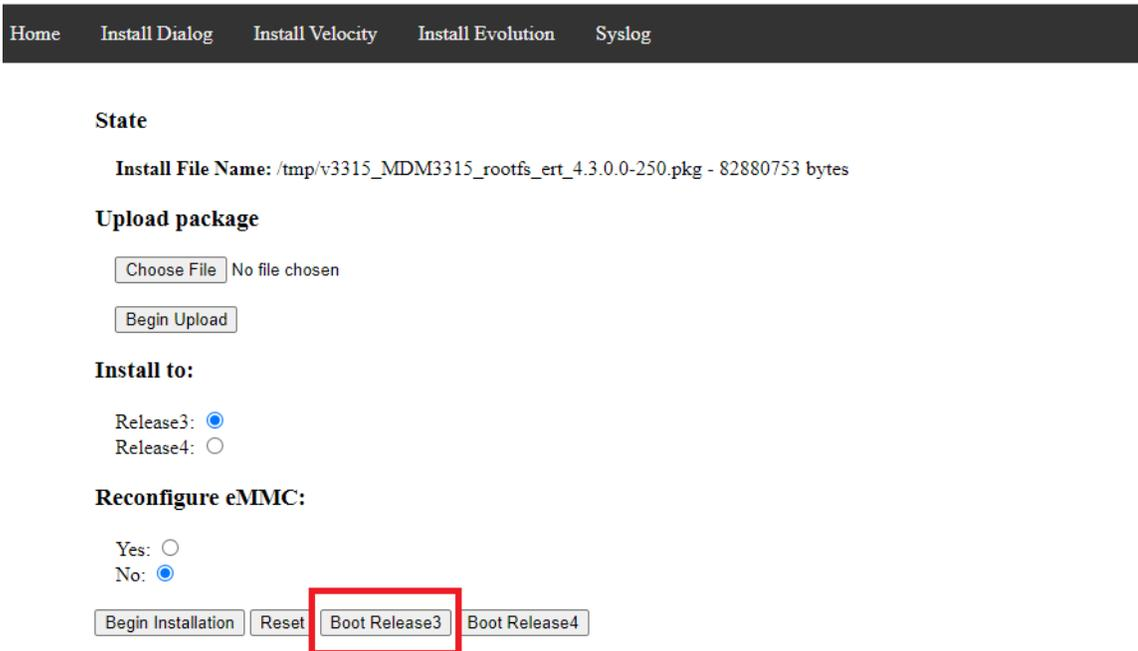
Figure C-14. Evolution Software Package Boot Release
