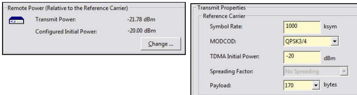
Figure 3-15. Initial Power in Probe and iBuilder
