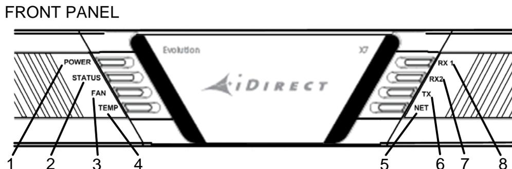
Figure 3-1. X7 Router Front Panel LED Display
