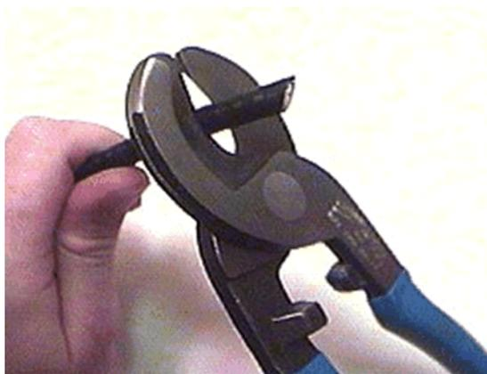
**Figure D-1. Coax Cable Cutting Technique**
