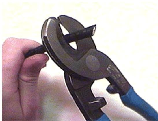
**Figure C-1. Coax Cable Cutting Technique**
