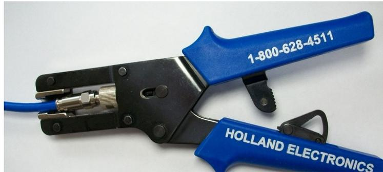
Figure C-5. Compression fitting F-Type Weatherproof Plug and Tool
