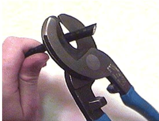
**Figure B-1. Coax Cable Cutting Technique**
