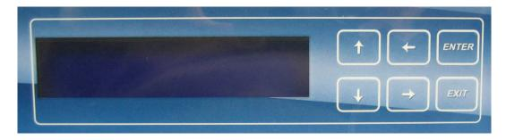
Fig. 13: iNetVu® 7000 Series Controller LCD and Keypad Navigator
