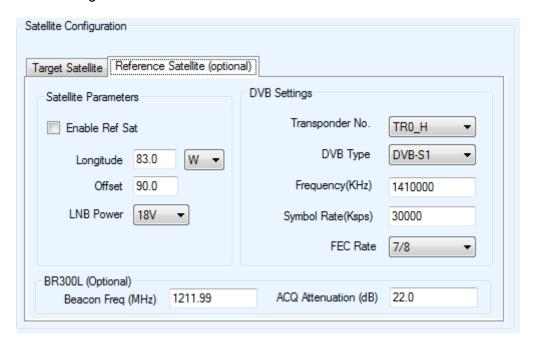
Fig. 90: Configuration – Reference Satellite Parameters
