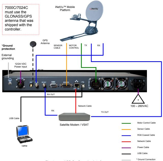
Fig. 4: USB Configuration Interface
