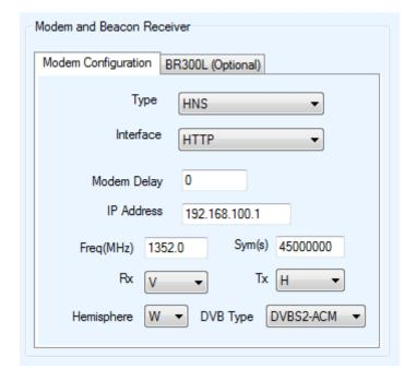
Fig. 91: Configuration – Modem Parameters
