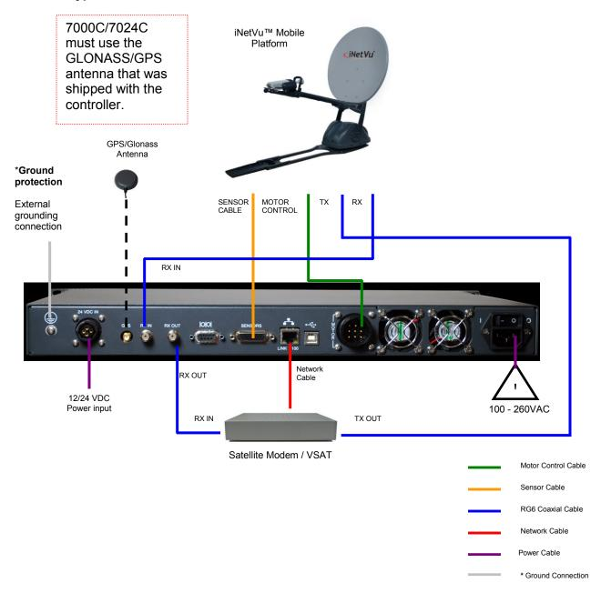
Fig. 6: *iNetVu*® 7000 Series Controller PC Free Connection Configuration
