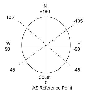
Note: Antenna reference point is 0° which means the reflector is pointing south with reference to the back facing North. The search window reference starting point will be the System Ref. AZ value, use above table and diagram to figure out which way the Antenna must be pointed (System Ref. AZ starting point) in order to set the AZ Window Size if an area is required to be excluded or blocked off from the search.
