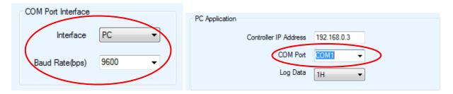
Fig. 9: Configuration for controller RS232 serial options
