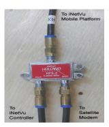
Fig. 34: RF Cable Setup for DIS selection
