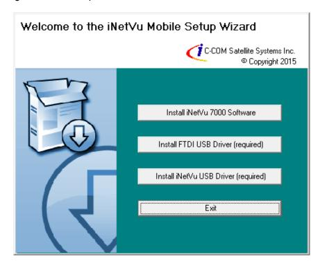
Note: The Driver installation will be done in two stages. FTDI CDM Drivers and, USB Drivers.
