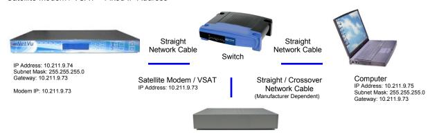
Fig. 117: Controller to Modem and PC network setup
