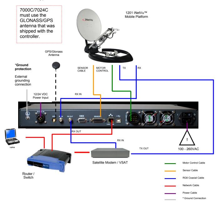
Fig. 3: iNetVu® 7000 Controller Typical Connection Configuration
