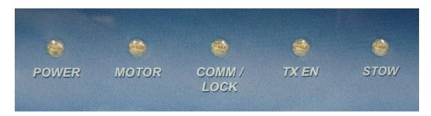
Fig. 11: iNetVu® 7000 Series Controller Front Panel LED Panel
