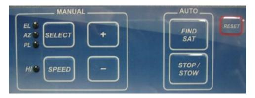
Fig. 12: iNetVu® 7000 Series Controller Front Panel Buttons
