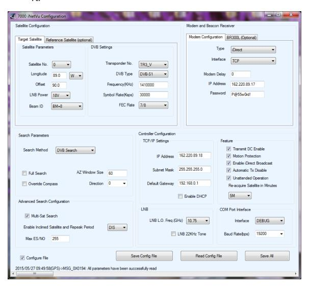
Fig. 87: iNetVu® 7000 Configuration Window
