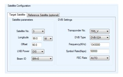
Fig. 88: Configuration – Satellite Parameters
