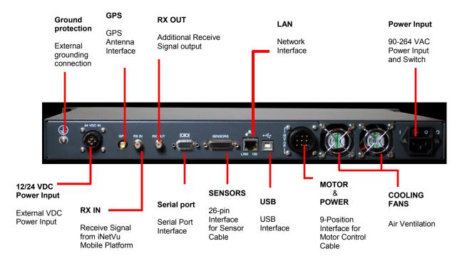
Fig. 2: iNetVu® 7000 Series Front and Rear Panel
