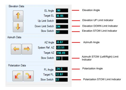
Fig. 68: Angle and Limit Switch Indicators
