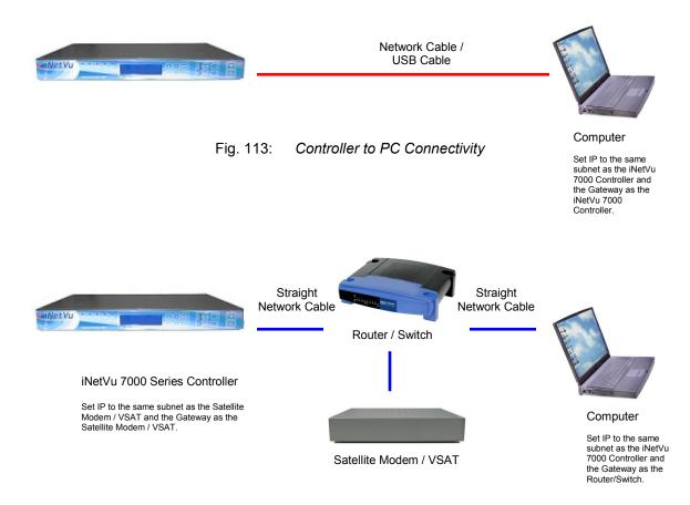
Fig. 114: Controller to PC and Modem Connectivity via Network Interface
