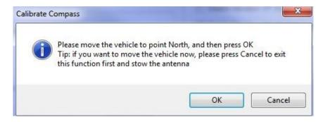
ii. Ensure that there are no metallic objects that could interfere with the Compass, and that the Mobile Platform is on level surroundings.
