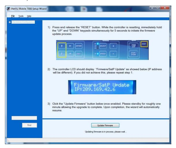
4. You may wish to continue through the wizard to complete the controller configuration or verify the settings. You can switch to the iNetVu software at any time by right clicking and selecting Controls.
