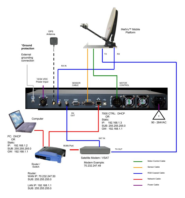
Note: VDC Power Input feature is available in the 7000C and 7024C Models Only. See Appendix for VDC power input external cable wiring.
