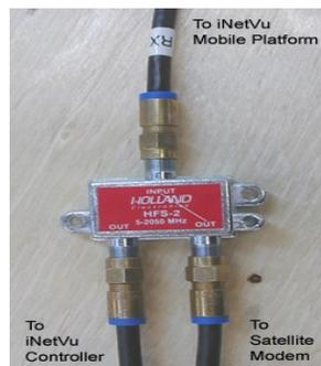
Fig. 39: *RF Cable Setup for DIS selection*
