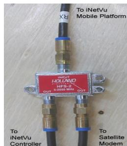
Fig. 89: RF Cable Setup for DIS selection
