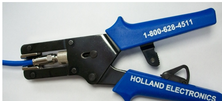
Figure C-5. Compression fitting F-Type Weatherproof Plugs and Tool
