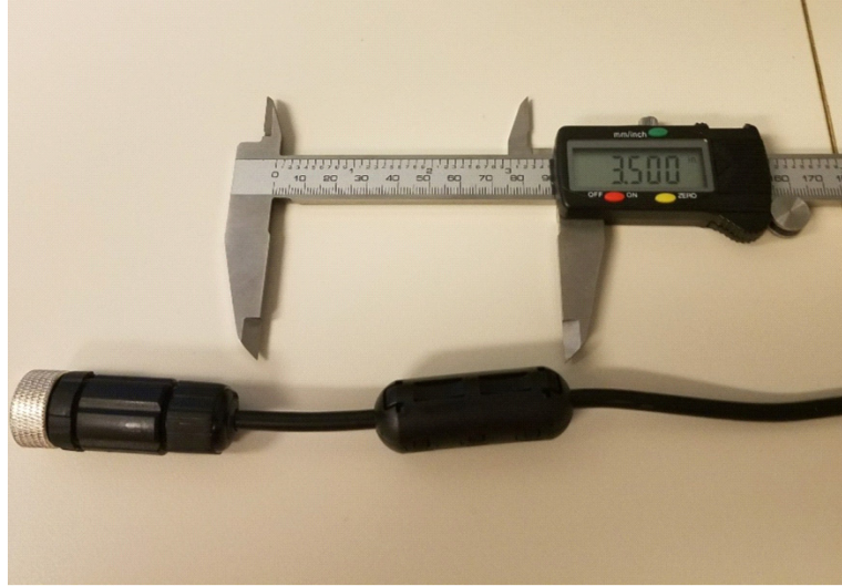
Figure 5-11. Ferrite Distance from the Rear
