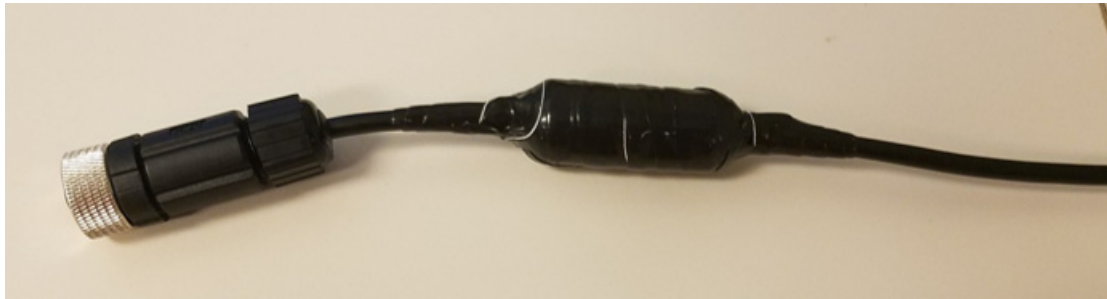
Figure 5-13. Ferrite Installation Complete
