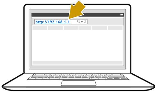
The first time your modem starts up, you are prompted for the Expert password in order to start the installation procedure. If your modem has already been installed before, you are re-directed to the Status page of the terminal.
