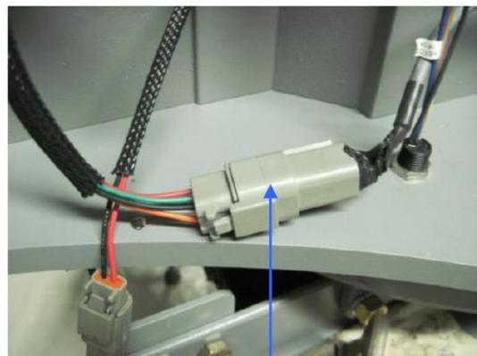
Azimuth motor connector
