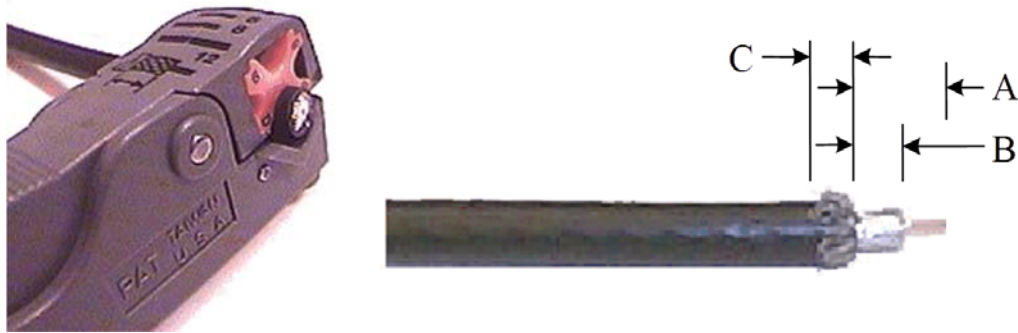
Figure 11. Cutting Technique for Removing Foil in the Braid
