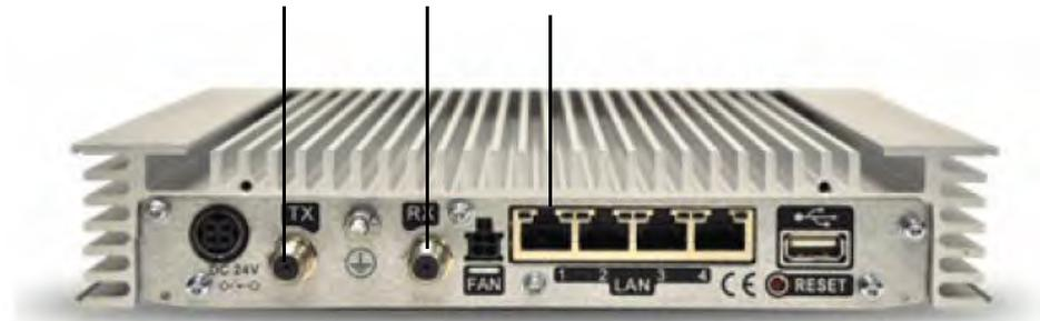
Figure C-7: Connecting Newtec MDM3100 to the ACU (OpenAMIP)
