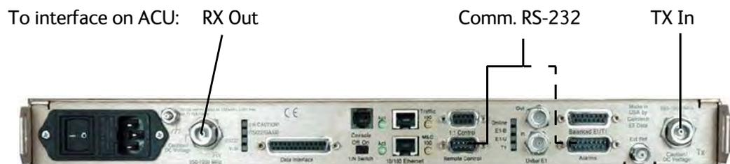
Figure C-14: Connecting COMTECH 570L to the ACU (example)
