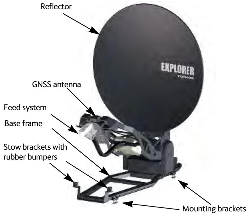
Figure 2-3: Antenna system components, part 2
