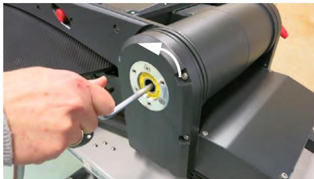
Figure 7-6: Manual elevation adjustment
