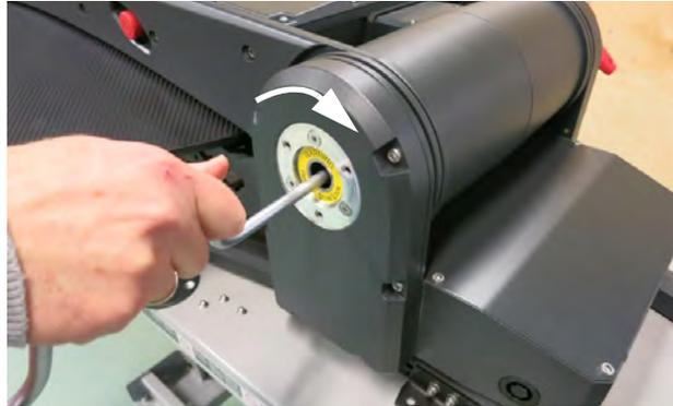
Figure 7-8: Manual elevation adjustment
