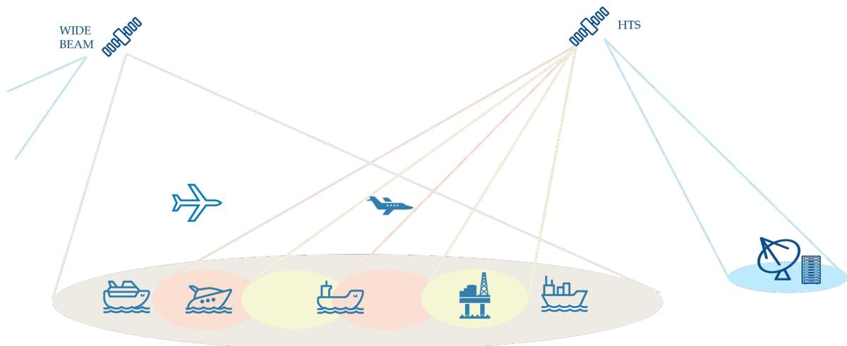
COTM terminals that can operate in multiple beams should have **Terminal Mobility**, **Automatic Initial Beam Selection (AIBS)** and **Automatic Pointing** enabled in the GUI.
