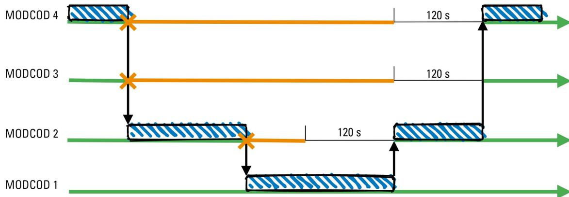
In the example we assume that, according to the ACM algorithm, the modem is able to use MODCOD 4. We also assume that at some point in time a local source of distortion appears, which degrades the forward link quality for the modem.
