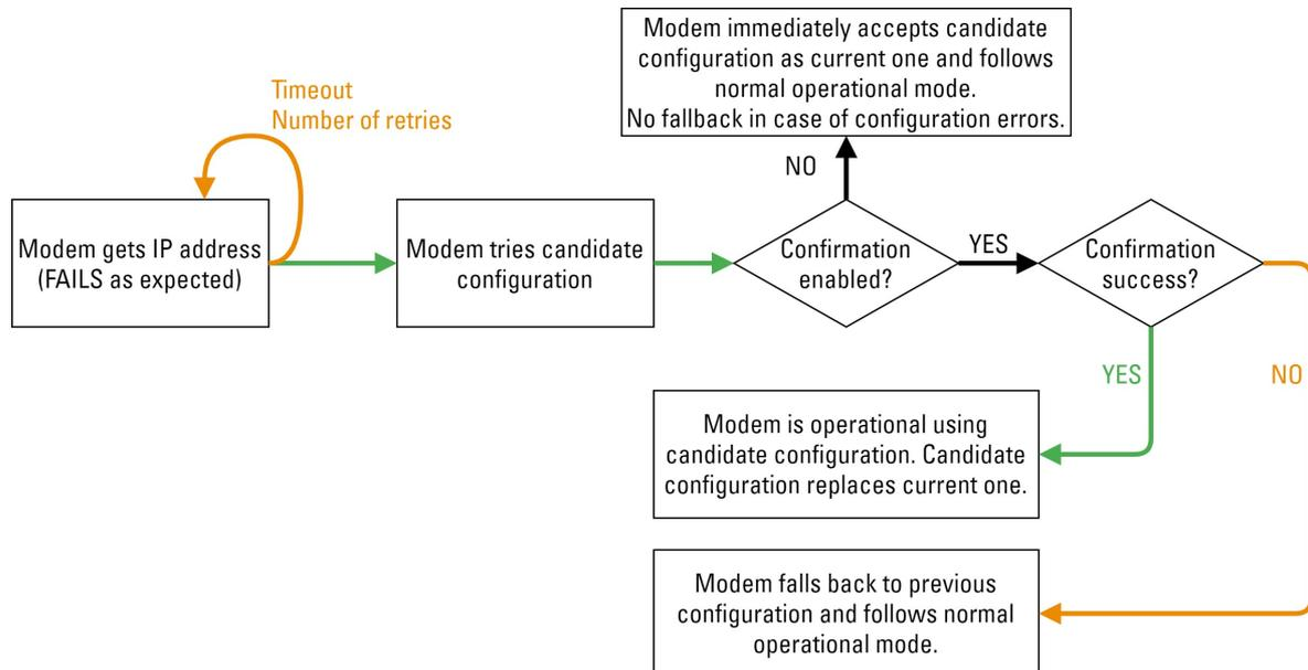
1. The modem tries to acquire an IP address from the DHCP server in the external network. As expected, this step will fail after timeout and a number of retries.
