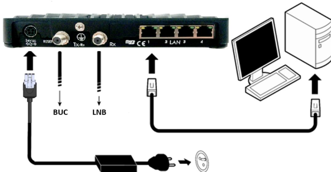
3. Make sure your computer is set to DHCP. Your computer will receive an IP address from the modem.
