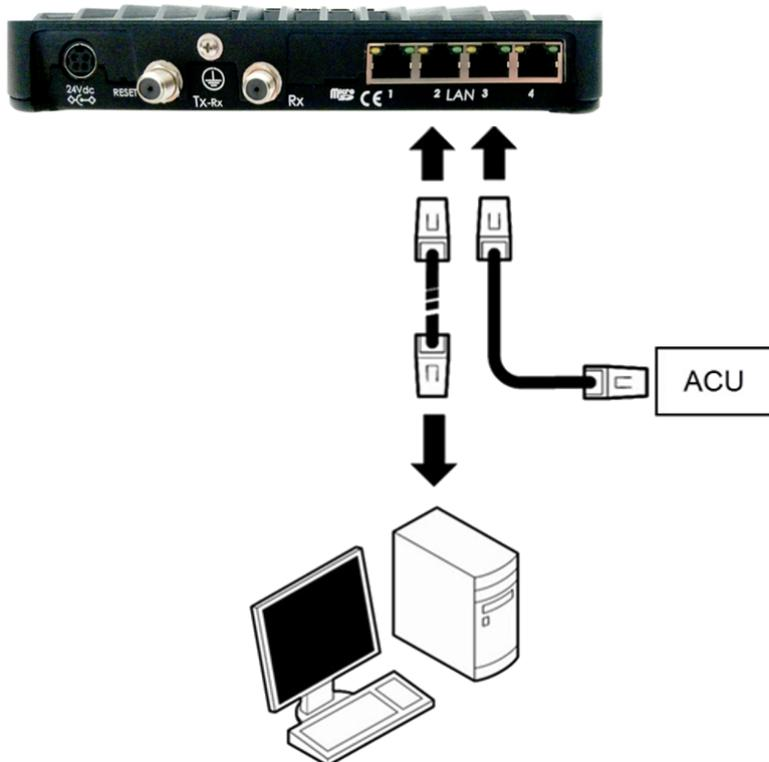
The modem and ACU communicate using OpenAMIP (Open Antenna to Modem Interface Protocol). The values for the parameters which are used for OpenAMIP communication between the modem and the ACU should be configured in the [Antenna Controlling on page 51](#) menu item. It is advised to click **Restart** after enabling automatic pointing.
