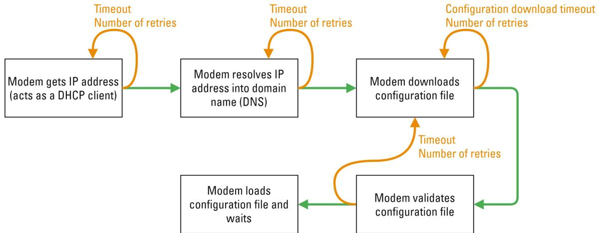
1. The modem acquires an IP address from the DHCP server in the LAN network.
