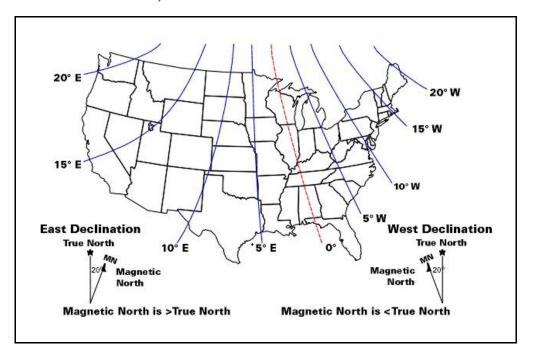
Figure 3-3. Example: Magnetic Declination
