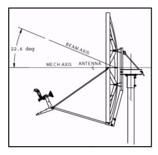
Figure 3-4. Antenna Elevation Offset
