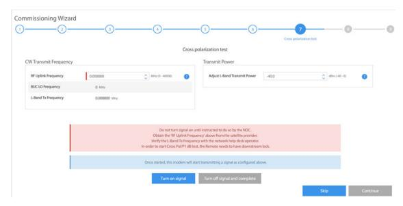
Figure 3-11. Cross Polarization test
