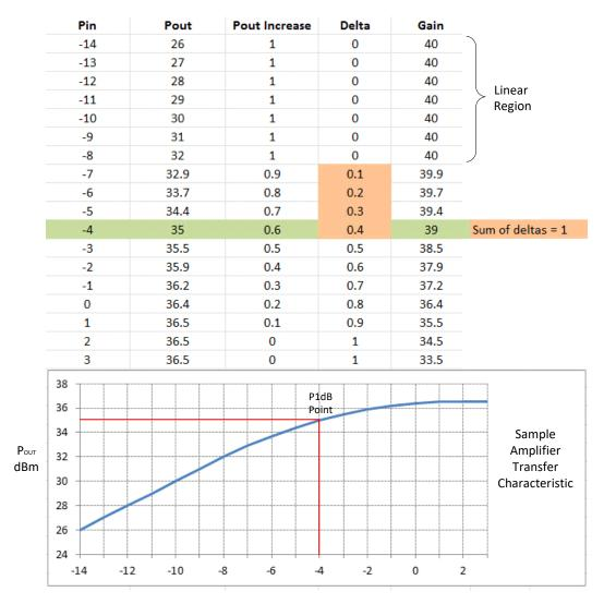
Figure 3-9. Sample Transfer Characteristic
