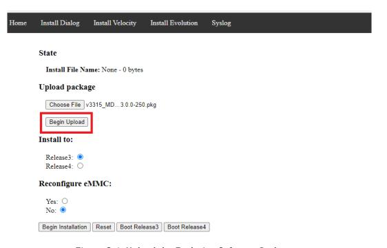
Figure C-4. Upload the Evolution Software Package
