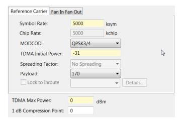
Figure 3-16. iBuilder Transmit Properties: TDMA
