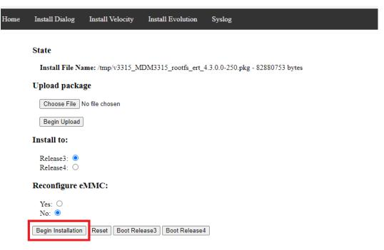
Figure C-9. Evolution Software Package Installation
