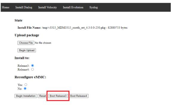
Figure C-14. Evolution Software Package Boot Release
