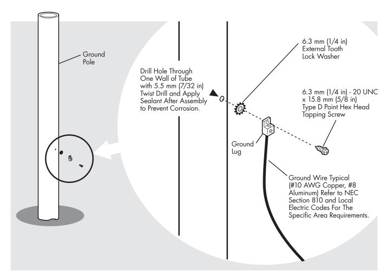
**NOTE:** All installations to conform to latest issue of National Electrical Code. Ground antenna mount assembly and feed cables in accordance with current National Electrical code and local codes.
