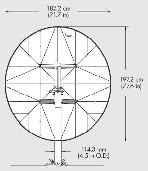
Type 183 1.8 Meter Offset Receive Transmit Antenna System
