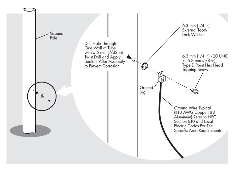
NOTE: All installations to conform to latest issue of National Electrical Code. Ground antenna mount assembly and feed cables in accordance with current National Electrical code and local codes.
