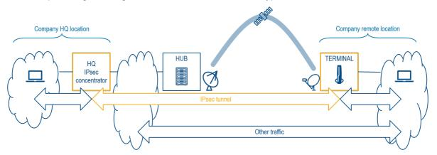
In case of multiple remote locations, a dedicated IPsec tunnel exists for each remote location. Communication between the remote sites always pass the headquarters.
