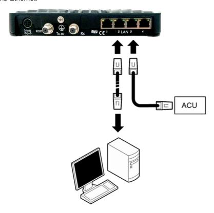
The modem and ACU communicate using OpenAMIP (Open Antenna to Modem Interface Protocol). The values for the parameters which are used for OpenAMIP communication between the modem and the ACU should be configured in the <a href="Antenna Controlling on page 44">Antenna Controlling on page 44</a> menu item. It is advised to click <a href="Reinstall">Reinstall</a> after enabling automatic pointing.
