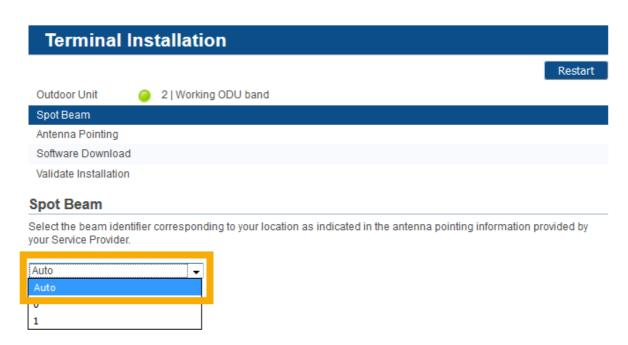
To select a beam, the terminal has to know its location on earth. Therefore, the **Antenna Control Unit** or **ACU** sends the GPS coordinates at regular intervals to the terminal using the OpenAMIP protocol.
