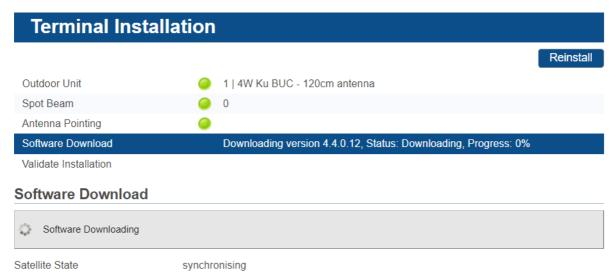
Once the download is complete, the new software is written to the flash memory and the modem reboots to activate the new software. You can now proceed with Validate Installation on page 27.
