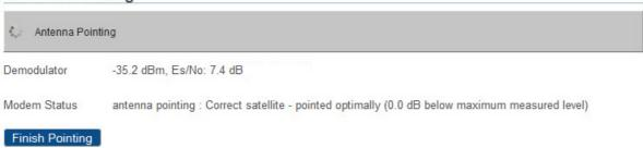
Pointing finishes automatically after the ACU has signaled to the modem that it has found the correct satellite.
