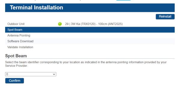
When using **automatic pointing** and **terminal mobility**, you can set the Spot Beam to **Auto**. This enables Automatic Initial Beam Selection or AIBS. With AIBS the beam is selected based on the GPS coordinates of the terminal and the beam contour information. You will see the extra installation state **Automatic Beam Selection**.
