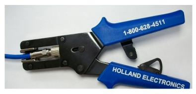
Figure C-5. Compression fitting F-Type Weatherproof Plug and Tool
