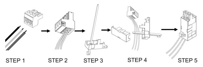
Figure D-1. DC-DC Power Supply Assembly at a Glance
