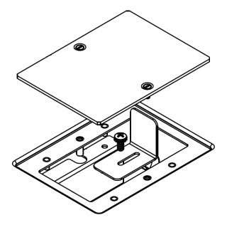
Figure 4-2. SIM Card Access Panel with L-Bracket
