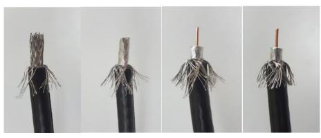
Figure C-3. Procedure to Cut the Quad Shield Cable
