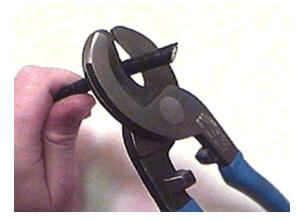
Figure C-1. Coax Cable Cutting Technique
