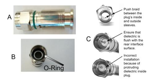
Figure C-4. Attaching the Compression fitting F-type Connector
