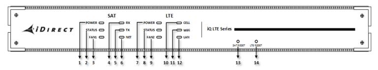
Figure 3-1. iQ LTE Satellite Router Front Panel LED Display
