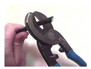
Figure B-1. Coax Cable Cutting Technique
