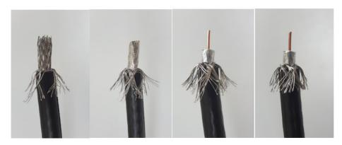
Figure B-3. Procedure to Cut the Quad Shield Cable
