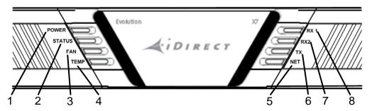
Figure 3-1. X7 Router Front Panel LED Display
