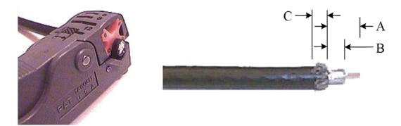
Figure D-2. Cutting Technique for Removing Foil in the Braid
